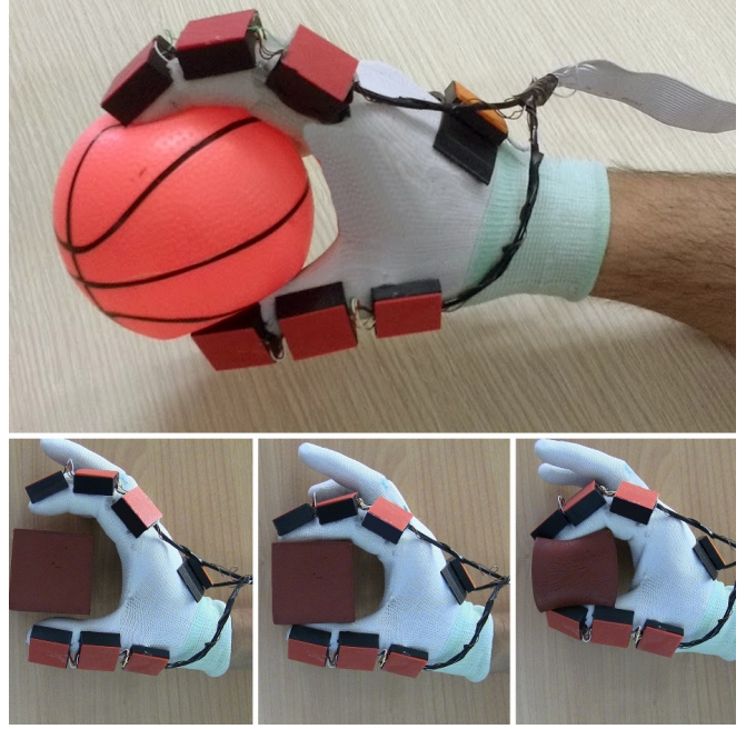
Fig. 1. Inertial and magnetic sensors can be used to estimate fingertip contact forces in grasping deformable objects: (top) a daily grasp situation, (bottom) a sequence of approaching, contact, and squeezing in grasping a deformable object.
